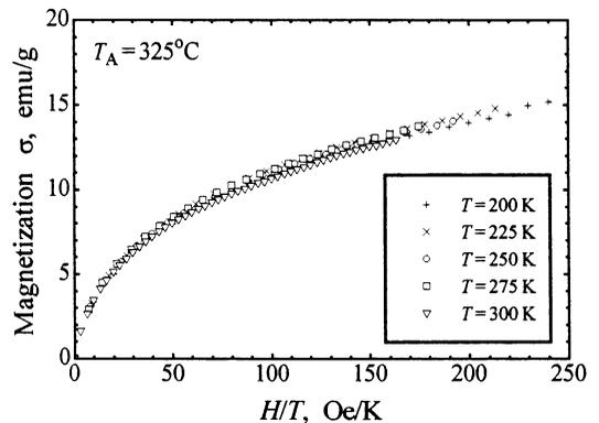
Fig. 8. Magnetization vs.  $H/T$  curves plotted at different temperatures for  $\text{CoFe}_2\text{O}_4$  powder annealed at  $325^\circ\text{C}$ .
