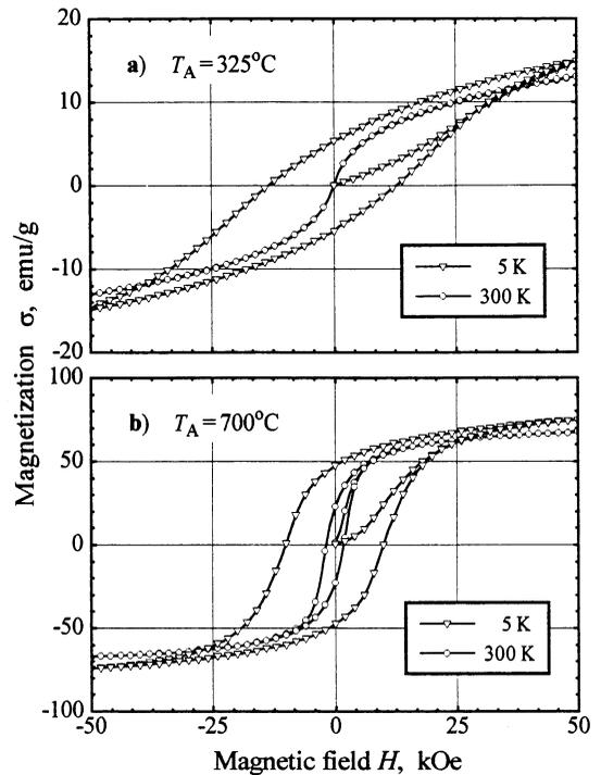
Fig. 7. Initial magnetization curves and hysteresis loops at 5 and 300 K plotted for  $\text{CoFe}_2\text{O}_4$  powders annealed at (a)  $325^\circ\text{C}$ , and (b)  $700^\circ\text{C}$ .
