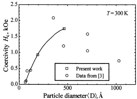
Fig. 11. Dependences of the coercivity at 300 K on mean particle diameter, and compared with the data reported in Ref. [3].
