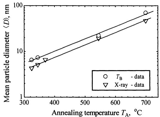
Fig. 2. Annealing temperature dependence of particle diameters estimated from broadening of X-ray diffraction peaks and from mean blocking temperatures.
