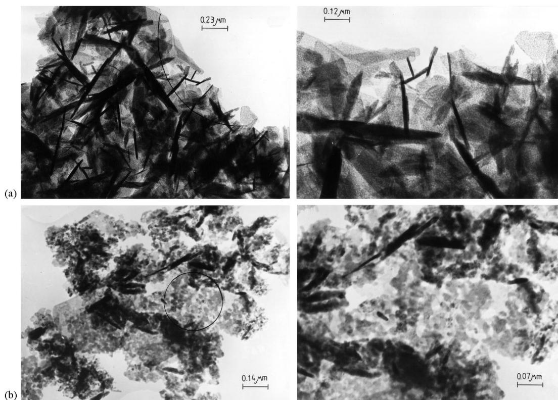
Fig. 3. Bright field micrographs of  $\text{CoFe}_2\text{O}_4$  powder annealed at (a)  $345^\circ\text{C}$ , and (b)  $545^\circ\text{C}$ . The pictures on the right-hand side represent the enlarged areas marked.
