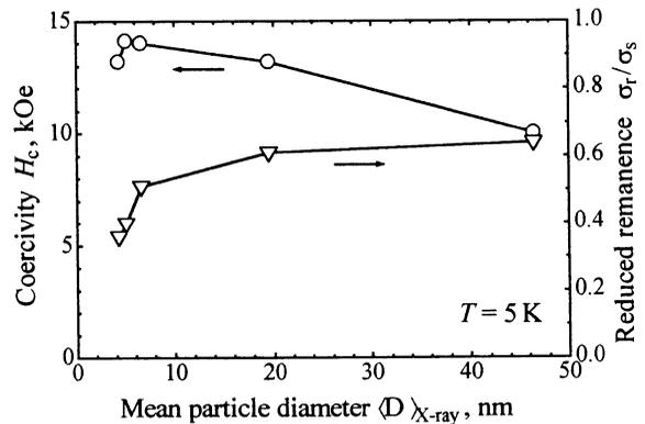
Fig. 9. Dependences of the coercivity and reduced remanence measured at 5 K on mean particle diameter.
