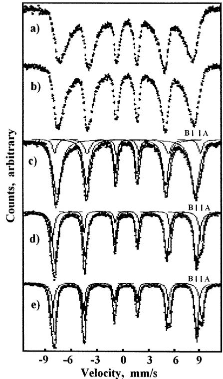
Fig. 5. Mössbauer spectra, obtained at 80 K for  $\text{CoFe}_2\text{O}_4$  powders annealed at (a) 325°C, (b) 345°C, (c) 370°C, (d) 545°C, and (e) 700°C.
