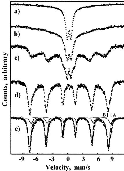
Fig. 4. Mössbauer spectra, obtained at 300 K for  $\text{CoFe}_2\text{O}_4$  powders annealed at (a) 325°C, (b) 345°C, (c) 370°C, (d) 545°C, and (e) 700°C.
