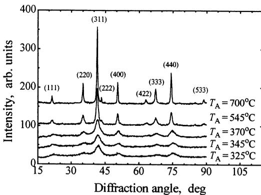
Fig. 1. X-ray diffraction patterns obtained using  $\text{CoK}_\alpha$  radiation of  $\text{CoFe}_2\text{O}_4$  powders annealed at different temperatures.
