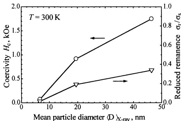
Fig. 10. Dependences of the coercivity and reduced remanence measured at 300 K on mean particle diameter.
