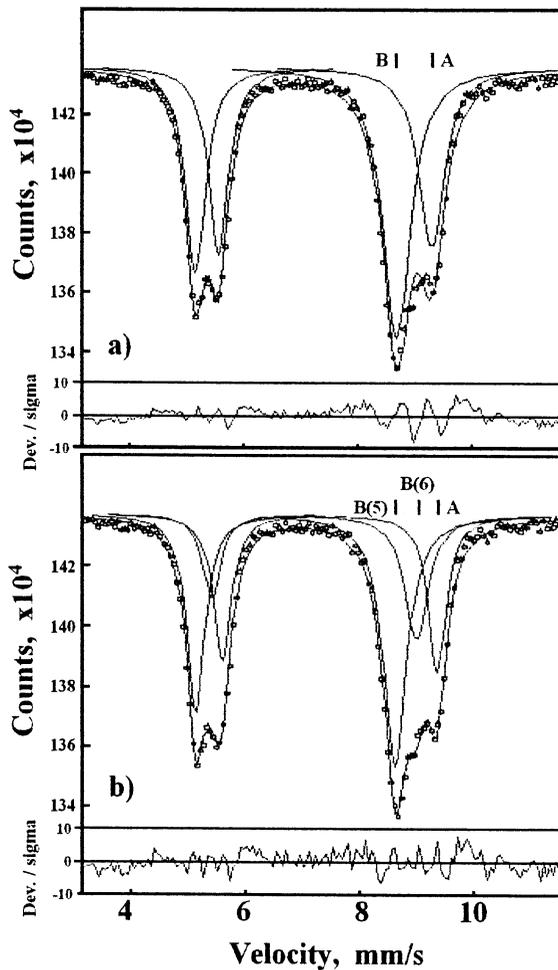
Fig. 6. Fifth and sixth Mössbauer lines obtained at 80 K for  $\text{CoFe}_2\text{O}_4$  powder annealed at  $700^\circ\text{C}$ , fitted with (a) two, and (b) three sub-lines.
